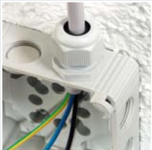
IP 65 with ADM 20 cable gland without locknut. The gland is secured by an integrated M 20 thread.
