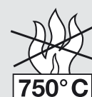
Burning behaviour: Glow wire test according to IEC 60 695-2-11: 750 °C, flame-retardant, self-extinguishing
