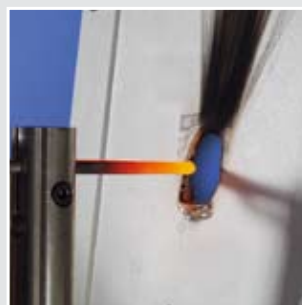
Burning behaviour: Glow wire test according to IEC 60 695-2-11: 750 °C, flame-retardant, self-extinguishing
