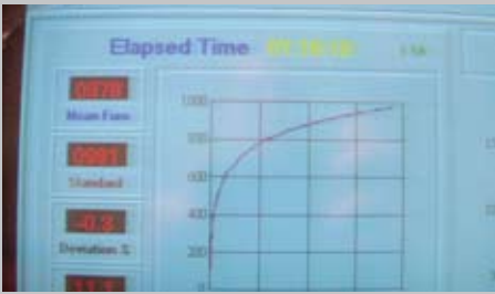
Test temperature curve in accordance with DIN 4102
